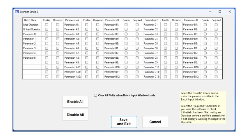
**Batch Processing Setup Screen:** Bar code scanning can be used to automate batch processes for quality requirements and to eliminated errors running profiles. You can have up to 56 parameters associated with each batch run.
