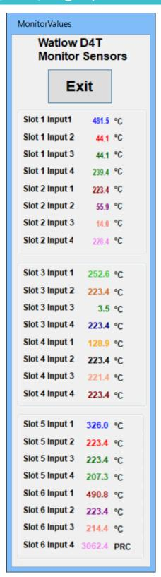
**D4T Monitor Screen:** 24 external sensors that can be data logged and viewed in the software. ProcessView supports an additional Watlow D4T that can be used to add up to 24 external sensors to a chamber or for a device under test.
