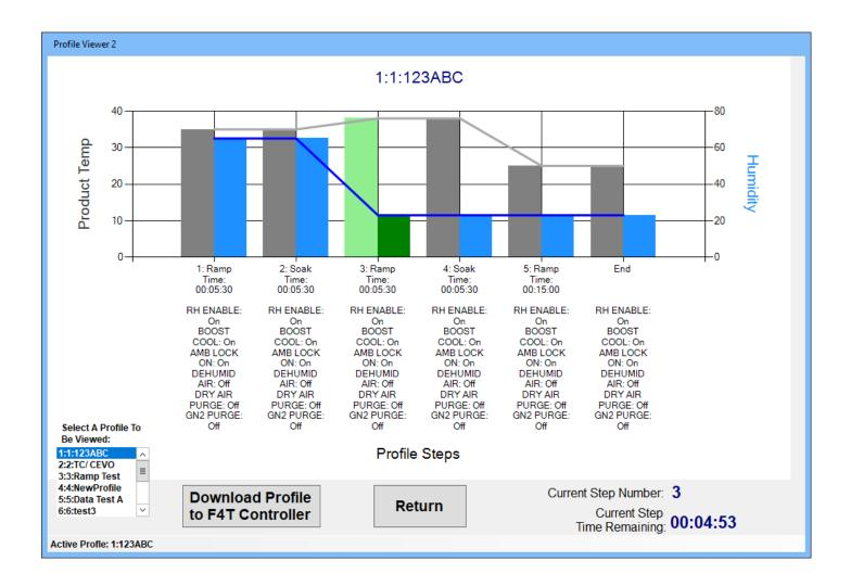
**Profile Viewer Screen:** Displays Selected Profile Graphically with Event Output status and if the profile is running the current step is shaded green and the current step number and timer remaining is shown.
