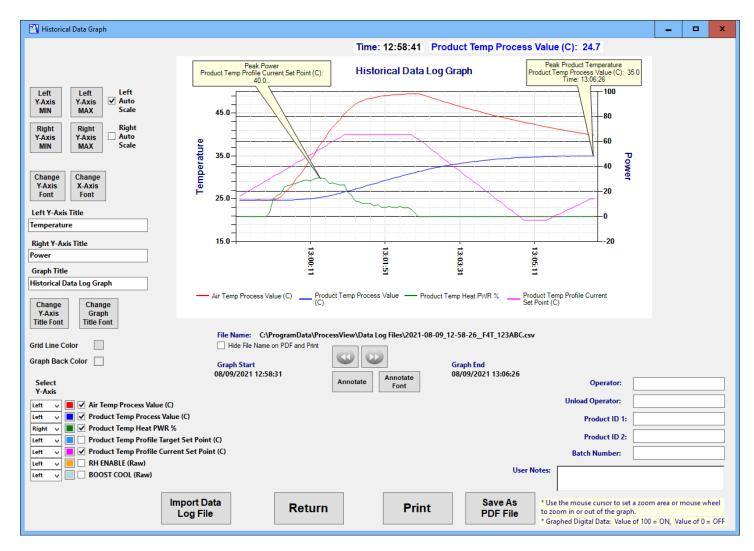
**Historical Data Graph Screen:** Saved data can be graphed for inspection and archiving purposes and saved as a PDF file or printed for a hard copy along with batch information. Annotation notes can be added on interesting or important data points. Axis Scaling and Batch information can be included in the saved graph.
