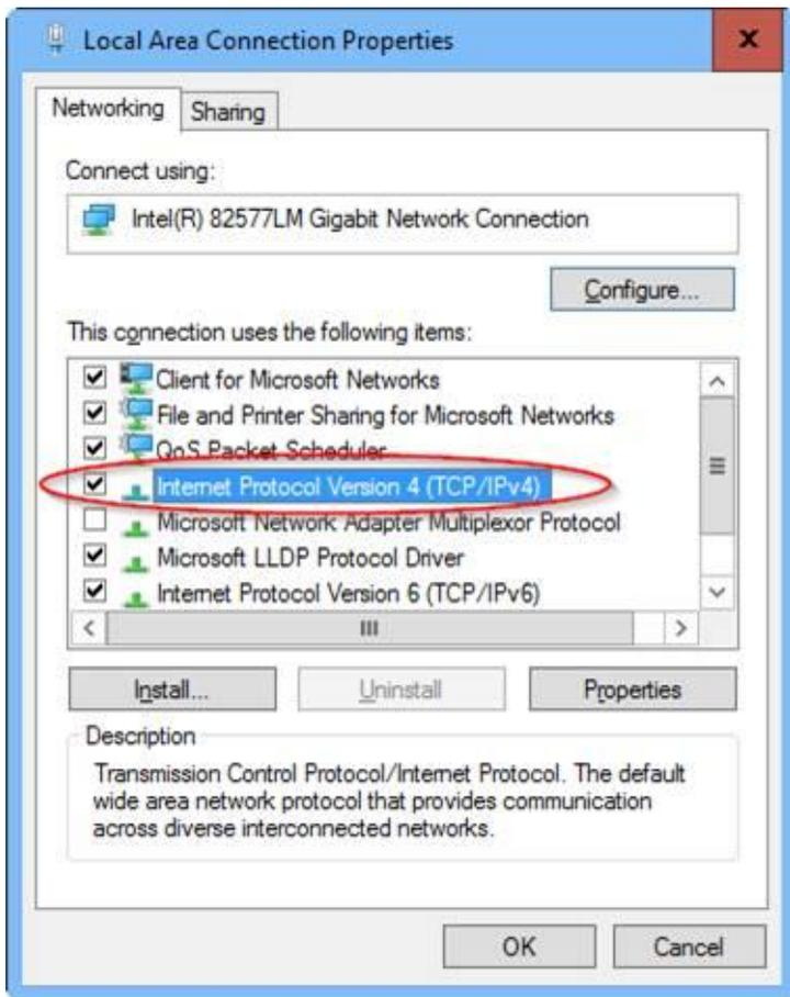
Then in the IP address field put in a network address that is on the same network as the F4T (Do not put in the same address as the F4T). The F4T default address is 192.168.0.222. If you put in an address that is something like 192.168.0.10 it will then be on the same local network. Make sure you select "Use the following address" as well. Enter 255.255.255.0 for the Subnet mask. Leave the Default gateway blank as show below:
