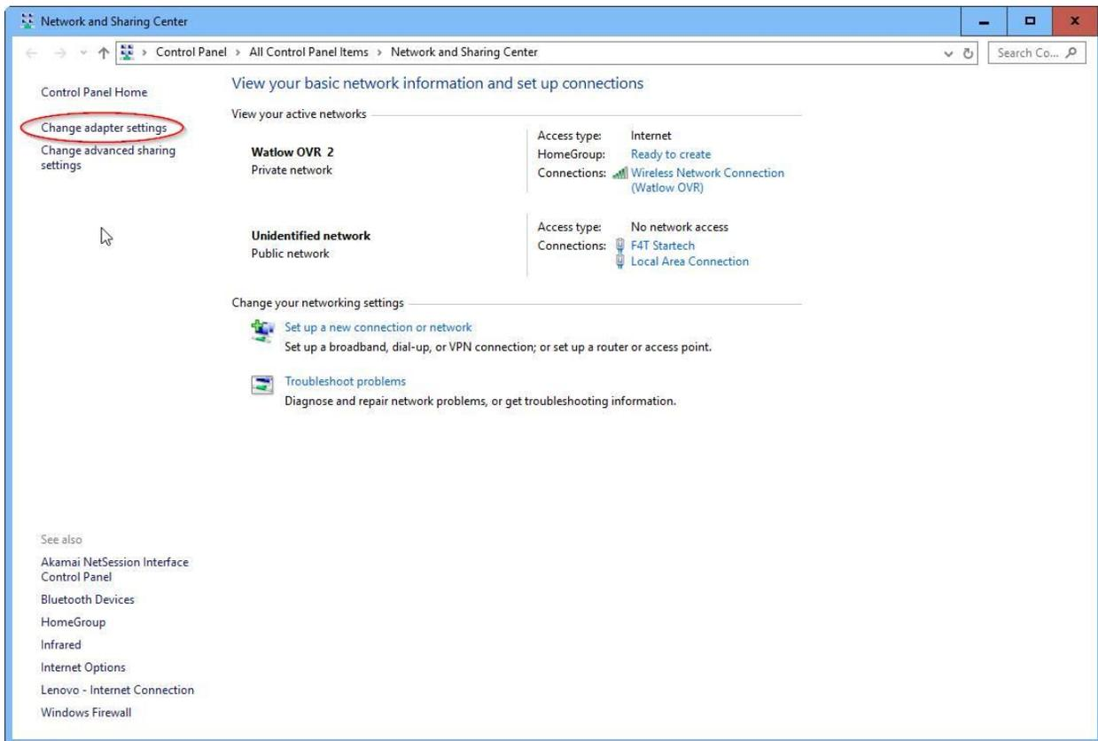
Then select the appropriate network adapter that is used to connect the Ethernet cable. If hardwired it will usually be the “Local Area Connection”. If wireless than select the “Wireless Network Connection”. Then “double click” on the selected network connection with your mouse.
